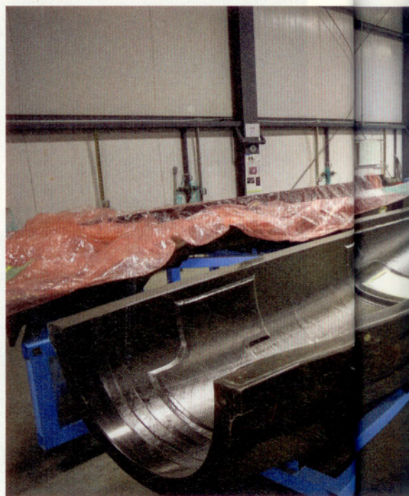
FUSELAGE MOLDS (above) allow the biggest pieces of the carbon-fiber airplane to be assembled and glued together like a model. Precise jigs (right) assure that the alignment of each airframe is close to perfect.
